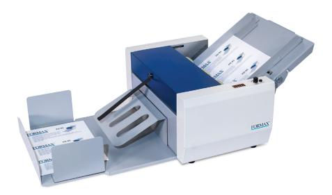
The **FD 95 Rotary Perforator/Creaser** is specially designed to finish printed sheets, up to 13.8" x 19". Its three-tire friction feeding system reliably feeds up to 7,080 sheets per hour, and can create up to 5 parallel perforations and/or creases in a single pass. Perforating allows for easy separation of multiple printouts, tear-offs, postcards or tickets on a single sheet, while creasing allows for easy folding and reduces unsightly cracking in digital printouts.
